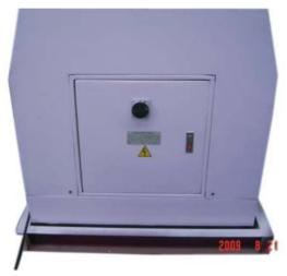
2)Press the START button on foot pedal controller, the motor starts up, hydraulic system is now ready to work. Press the emergency stop button down, the motor stops and hydraulic system also shuts off.
