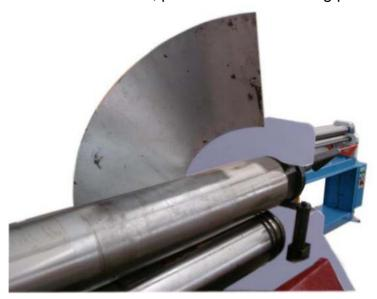
Press the yellow button and black button to adjust the rear axle and upper roller level until the distance could clamp the material tightly at the shorter side.
