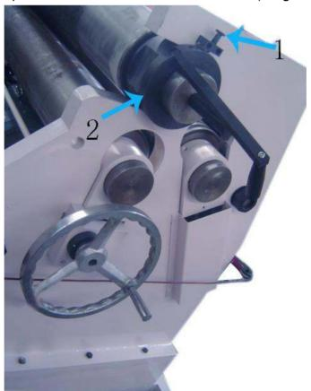
Put the steel plate through upper roller and front lower roller
