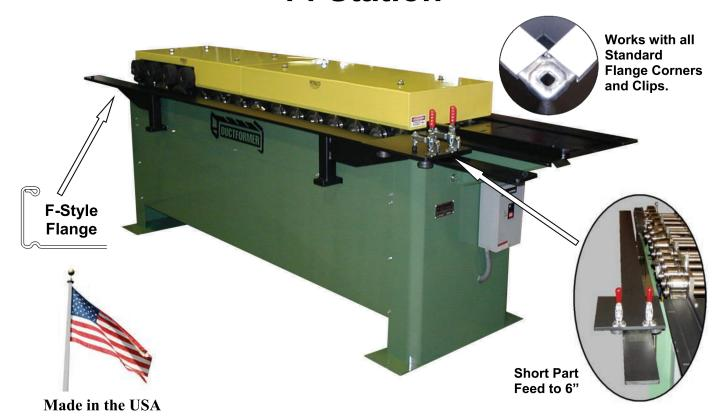
Ductformer's TDFC Rollformer comes with Edge Form Flange Rolls and Short Part Feed Roller Track. The Flange can be formed on Straight Duct and Fittings utilizing Standard Corner Flanges and Clips. The TDFC Design Simplifies Fabrication of Medium and High Pressure Duct.
