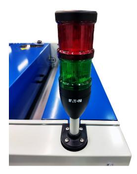
The AutoKut 1250 has a light tower to alert the operator which mode the machine is in. Standby, manual and run modes are all visible from a distance. This helps ensure a safe environment around the machine and shop. The material can be easily seen from the top of the slitter knife housing through two clear panels.
