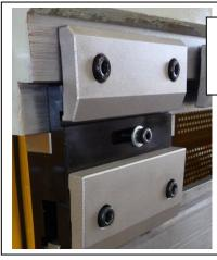
Our **optional** ram clamps for all punch Tangs shown above. Lever action allows for quick tool change.
